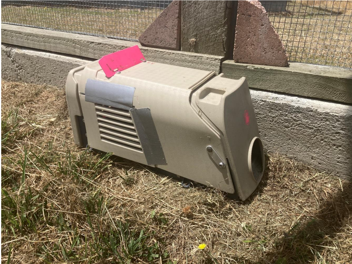
Figure 1. Unset Rewild kill trap deployed in observation pen. The raised pink flag on top of the trap indicates that the trap is unset or has fired. The trap was baited with a combination of chicken mince, dog roll, and cat biscuits placed in the bait well of the trap, located behind the trap treadle at the rear of the trap (not visible).
