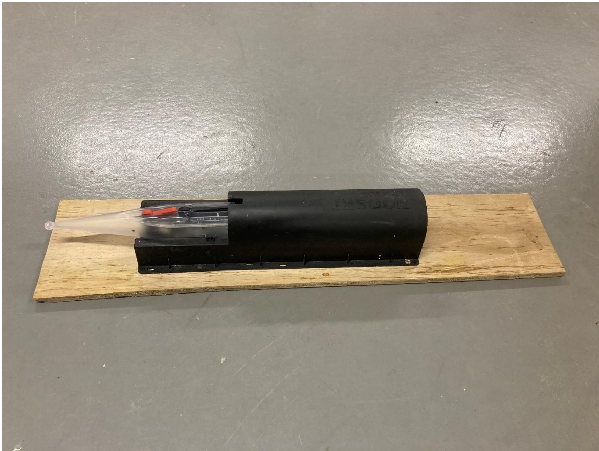
Figure 11. Nooski rat trap as deployed for testing. The trap was screwed to a 7mm plywood board to increase stability.
