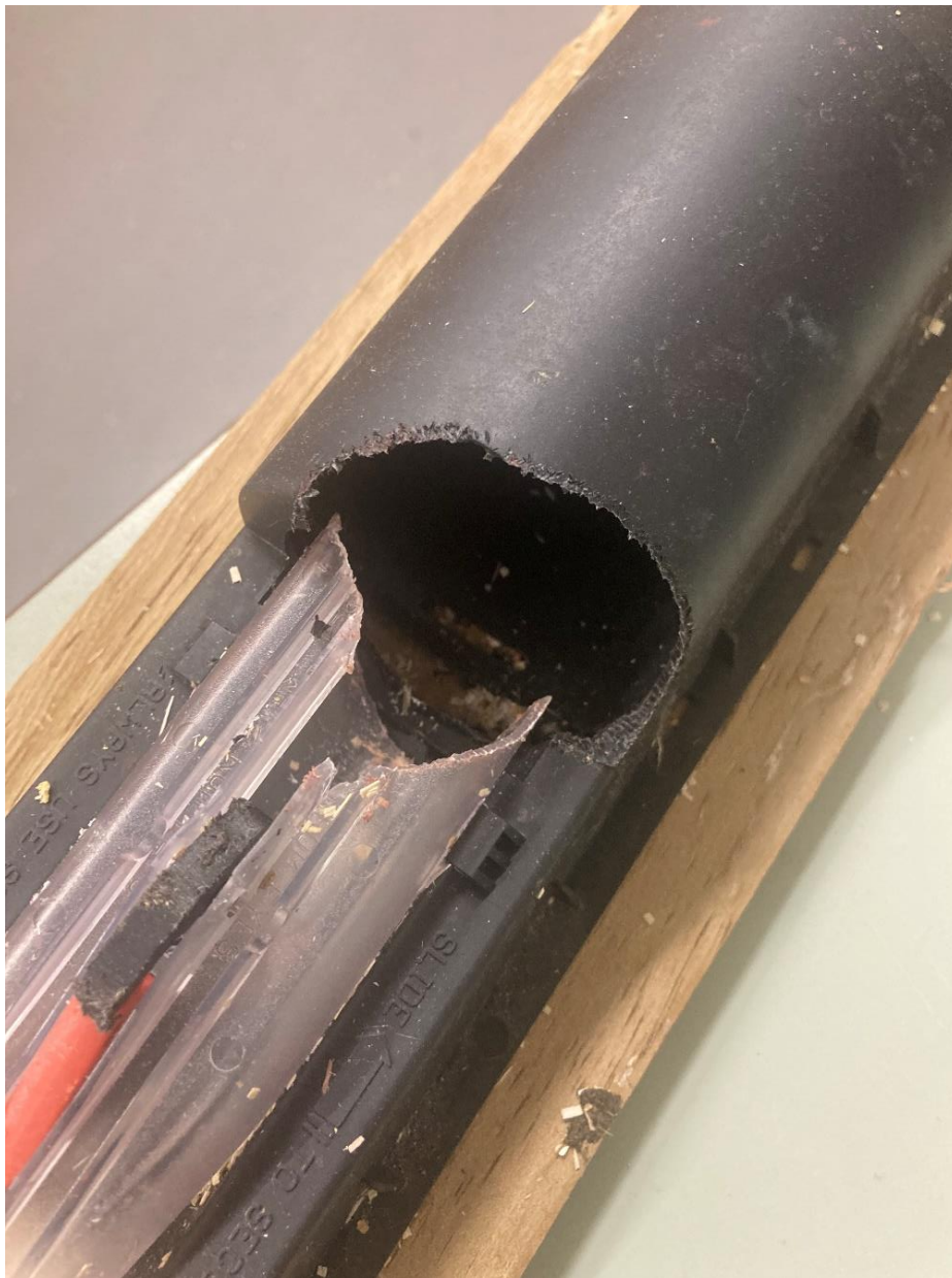
Figure 16. Nooski rat trap with gnawing damage from a Norway rat after being left unset during the acclimatisation and pre-feeding period.
