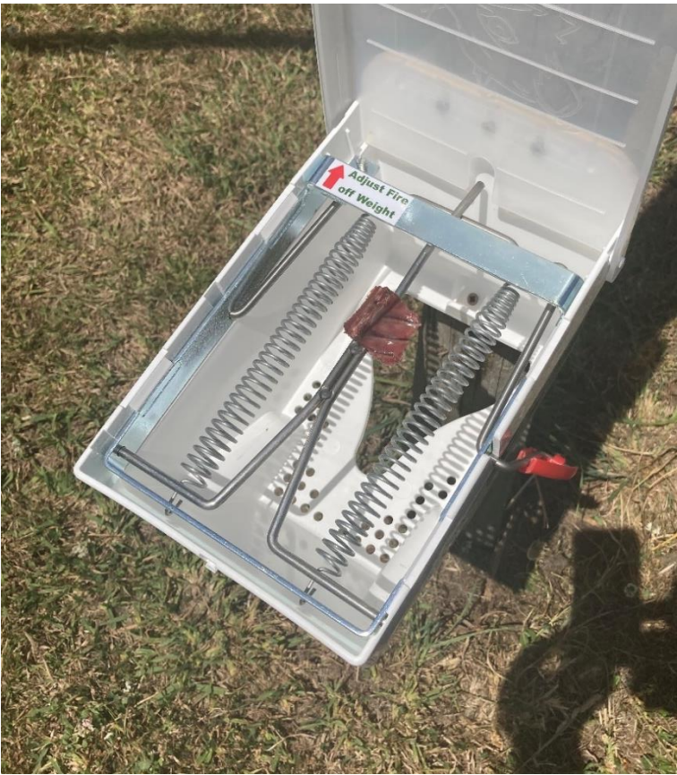
Figure 6. Set Trapinator kill trap showing position of rabbit meat bait. This photo was taken during initial non-lethal testing when the trap was secured 45 cm above the ground.
