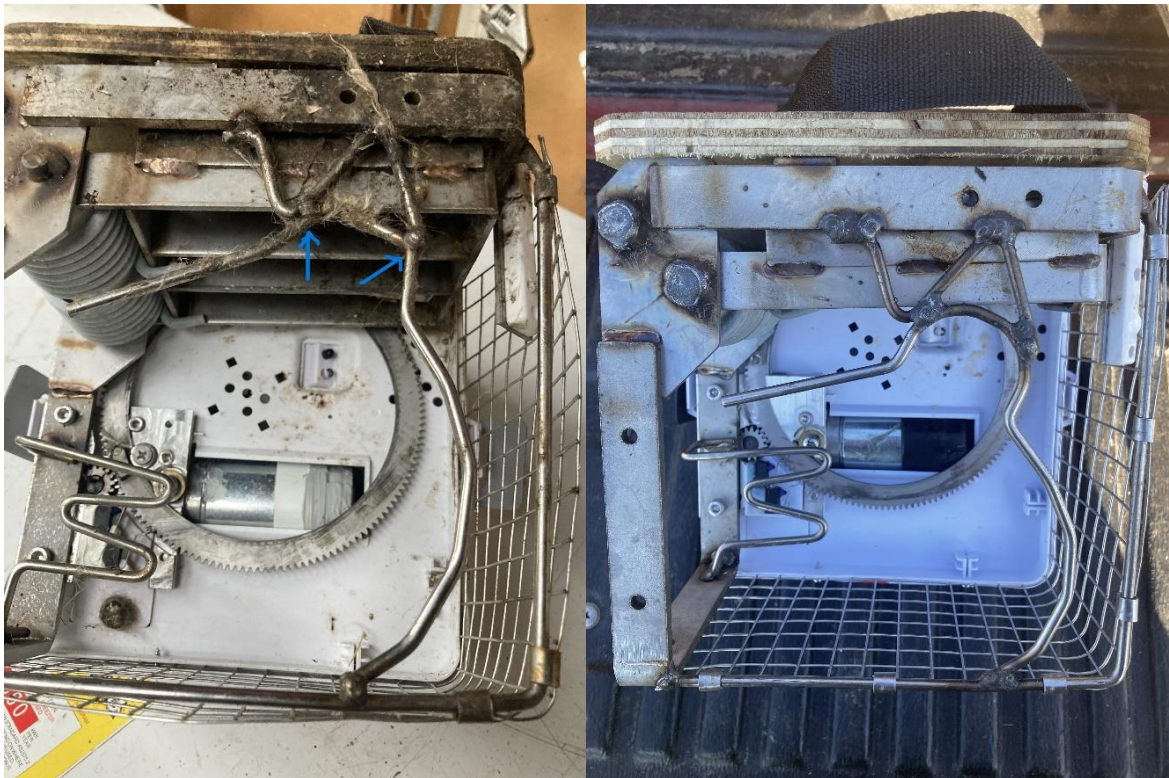
Figure 7. Underside of unset AT220 kill traps showing keyhole position. Blue arrows indicate corners in the original keyhole design (L), which were removed for trial 2 (R).
