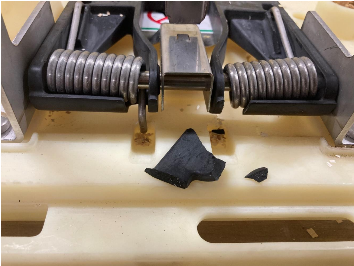
Figure 14. Springs of Trapinator Fusion kill trap, with broken parts that were previously encasing the underside of the right spring.
