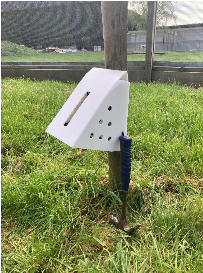
Figure 2. Sentinel trap as deployed for Test 2. The top of the trap (obscured by the coreflute cover) was 50 cm above the ground.
