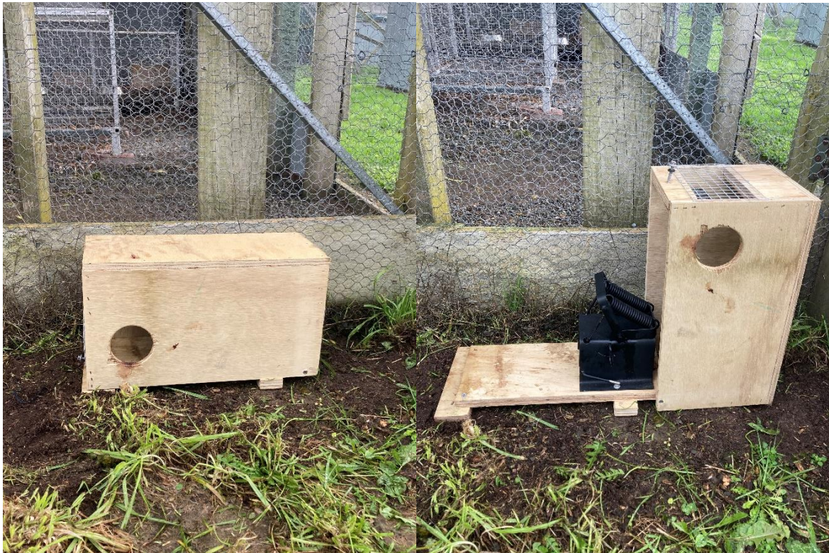
Figure 10. Unset SA4 trap deployed in an observation pen. The trap tunnel has mesh front and rear and 70 mm diameter entrances on each side (L). The tunnel cover was secured with a hex-head screw to the base. The screw was loosened to pivot open the tunnel cover (R) to access the trap and assess captured ferrets. The trap was baited with a cube of rabbit meat secured on a bait spike at the rear of the trap (not visible).
