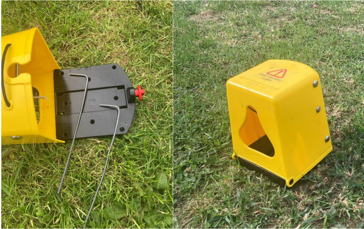
Figure 4. Flipping Timmy trap used for Test 3. Two 20 cm pins were used to secure the trap to the ground. The trap was baited with a piece of rabbit meat impaled on the trigger rod.
