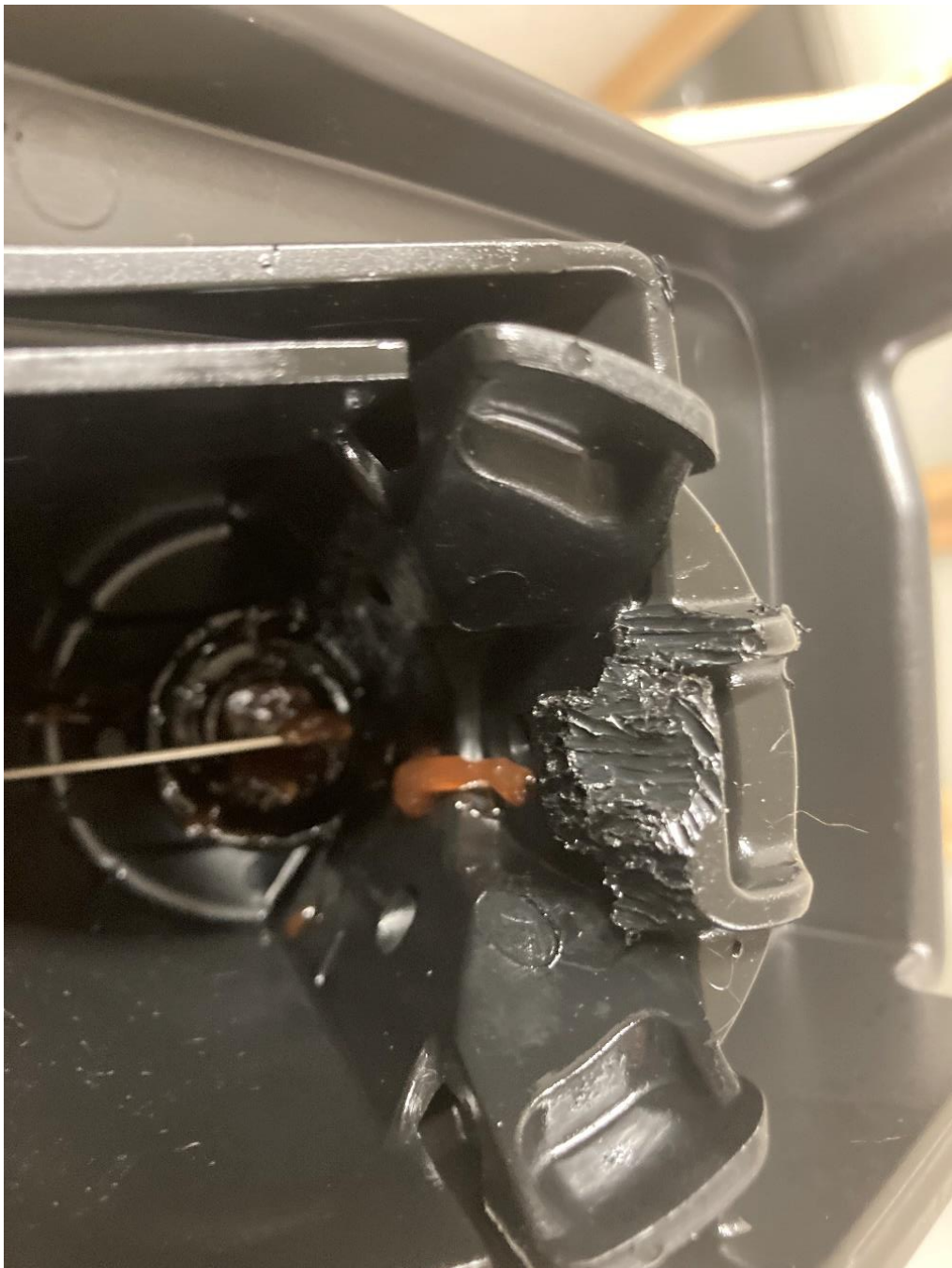
Figure 13. Underside of A24 kill trap showing Norway rat chewing damage on anvil. Note that chocolate-based rodent paste has dripped down the inside of the trap.
