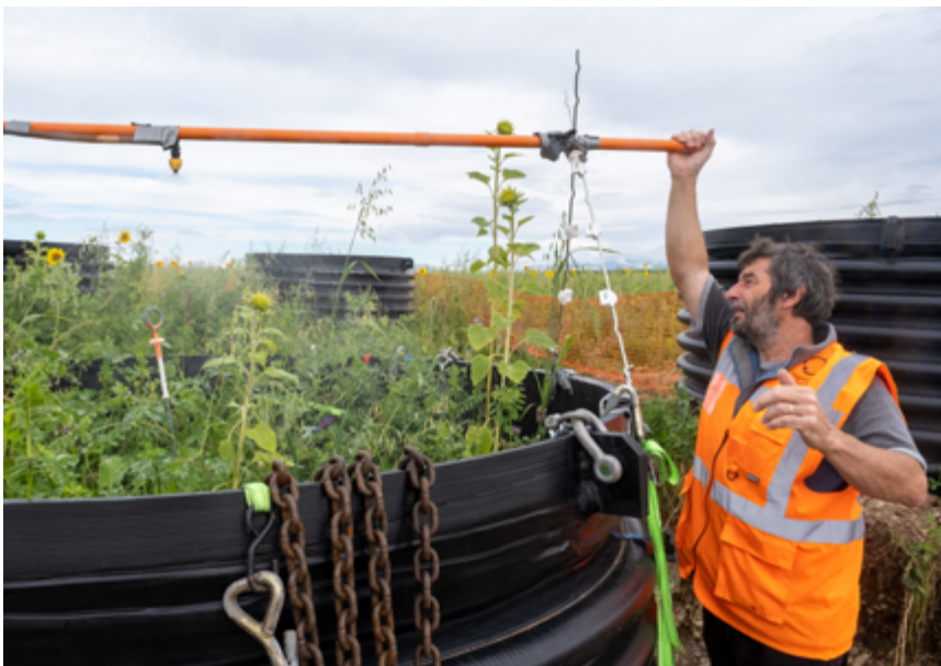
Research technician Graeme Rogers at the lysimeter installation for Te Whenua Hou, Te Whenua Whitiara. Image: Kim Triegaardt.
